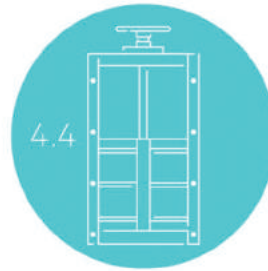
Non-Rising Stem Weir Gate
